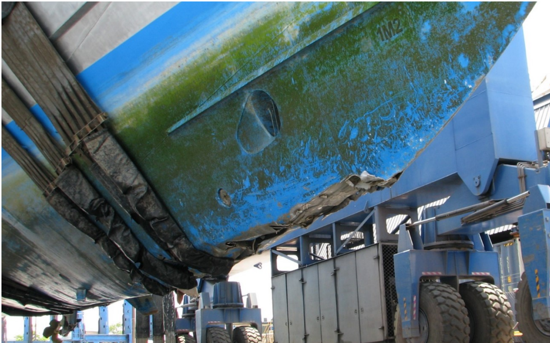
Figure 9: Damage to ABFC Roebuck Bay's keel
