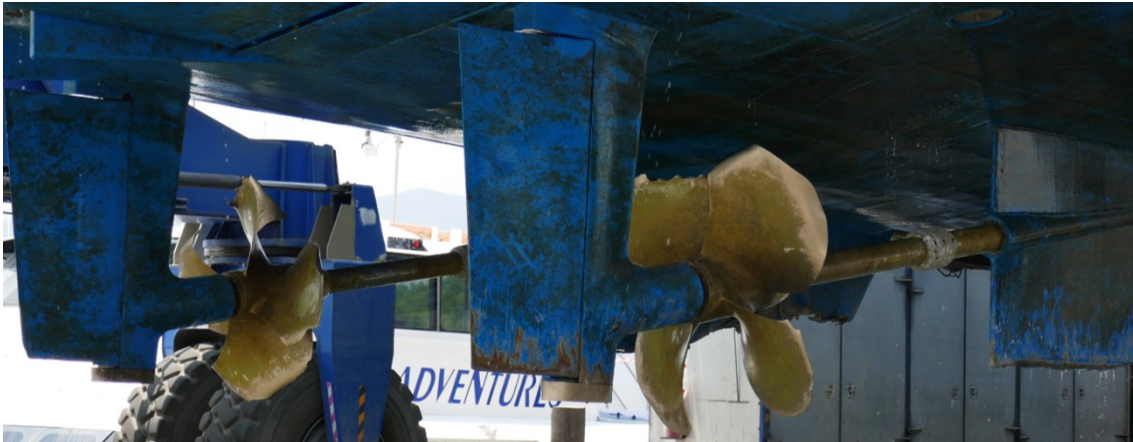
Figure 10: Damage to ABFC Roebuck Bay's propellers, rudders and skegs
