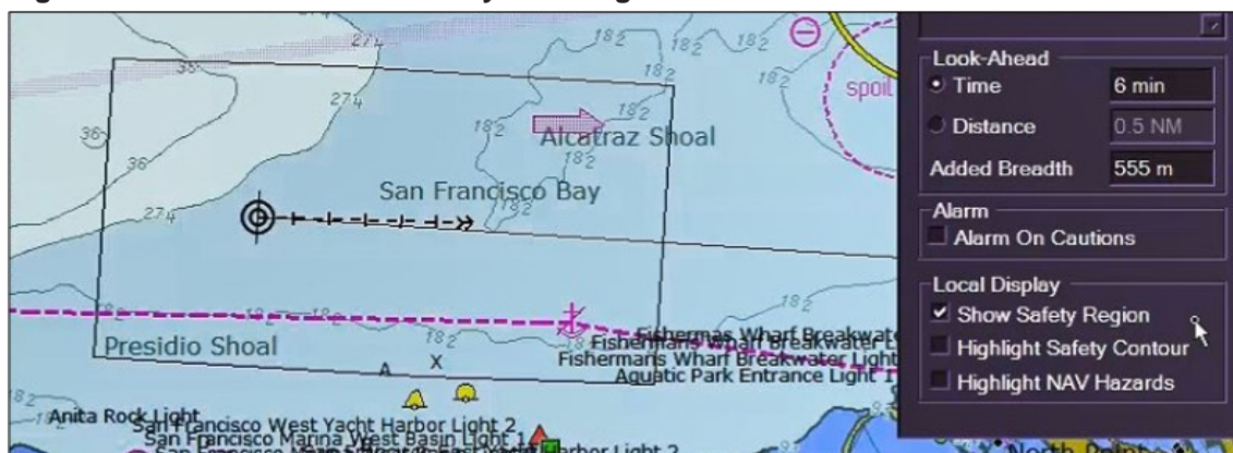
Image shows the key settings of the look-ahead safety checking function on a VisionMaster FT ECDIS. The rectangle represents the safety region 'box'. Source: Safebridge
