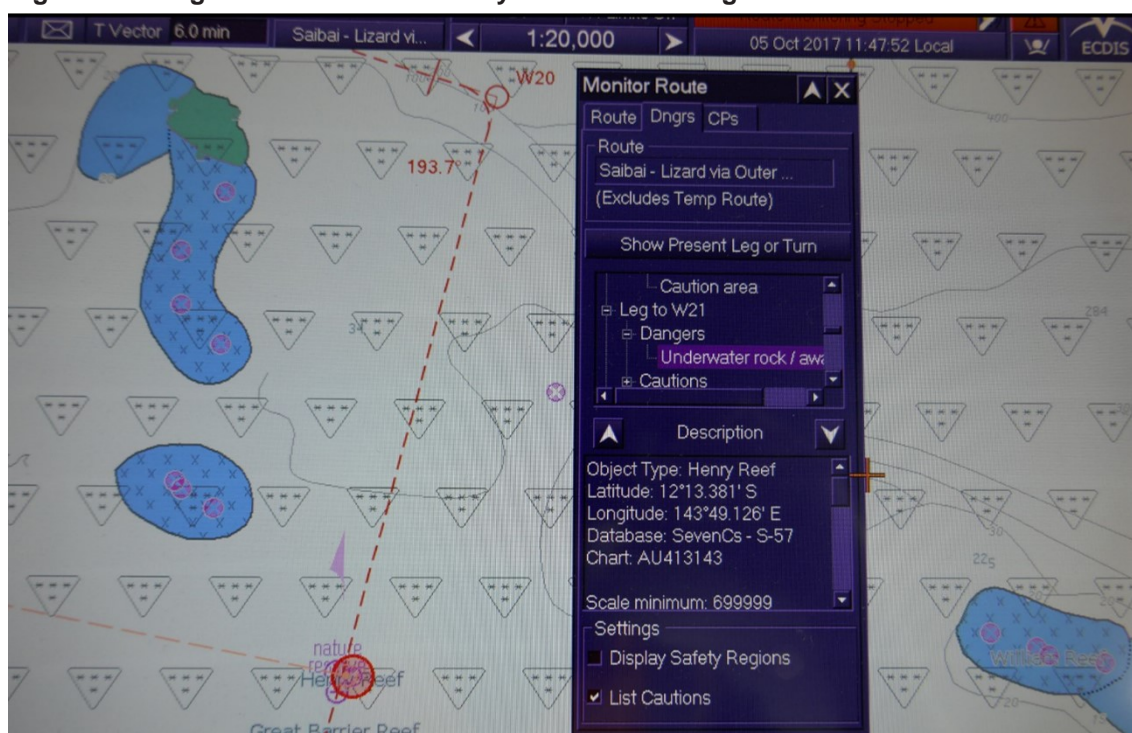
Image of ABFC Roebuck Bay’s ECDIS showing an identified danger (Henry Reef) on the leg to W21 in the dangers tab folder of the ‘Monitor Route’ window. Selecting the danger highlights the reef graphically on the ECDIS display and provides available information on Henry Reef. Source: ATSB
